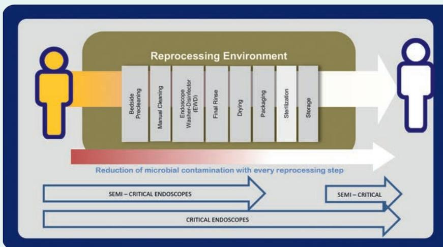
Figure 1: Reprocessing Steps for semi-critical and critical endoscopes
